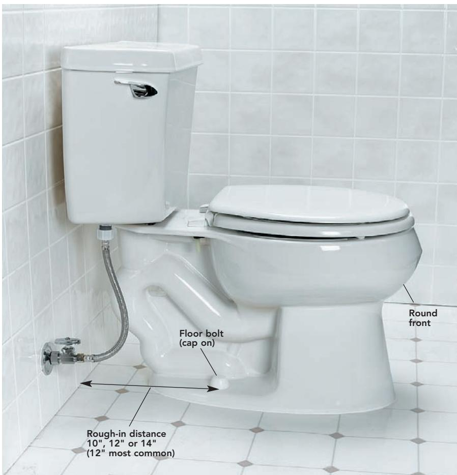
Buy a toilet that will fit the space. Measure the distance from the floor bolts back to the wall (if your old toilet has two pairs of bolts, go by the rear pair). This is your *rough-in distance* and will be either 10" or approximately 12". Make note of the *bowl shape*, round or oval (long). Oval bowls (also called elongated bowls) are a few inches longer for greater comfort, but may be too big for your space. The safest bet is to buy a replacement with the same bowl shape.
